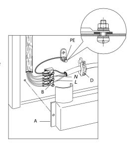
Figure 16a Connecting the feeder cable
